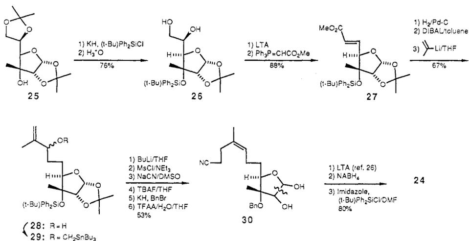
(enantiomerically pure) *Z*-homoallylic nitrile **24** was required. We have found that this compound can be prepared from *D*-glucose (Scheme VII).
